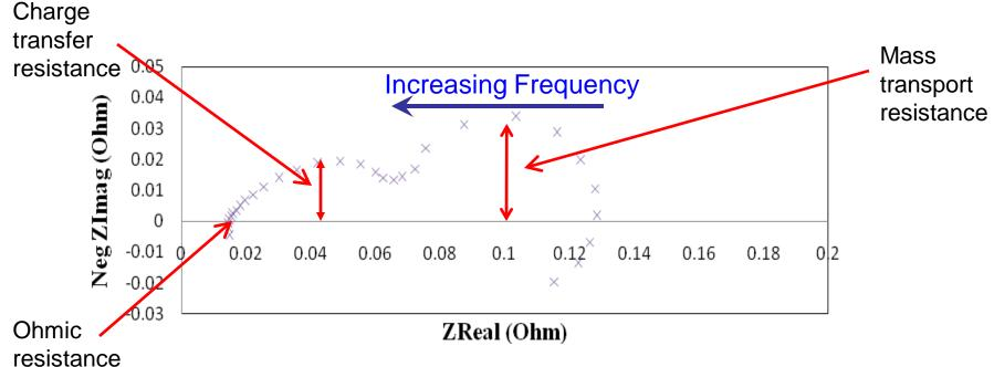
Typical Nyquist plot obtained in the present study. This particular one is generated under a anode 95%RH, cathode 95%RH, 1.5 cathode stoich, 2.5A (0.1 A/cm<sup>2</sup>) DC current.
