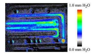
Neutron Imaging Technique. From Satija, R. et. al. *Journal of Power Sources*, 129, 238-245. Contributes to parasitic power losses
