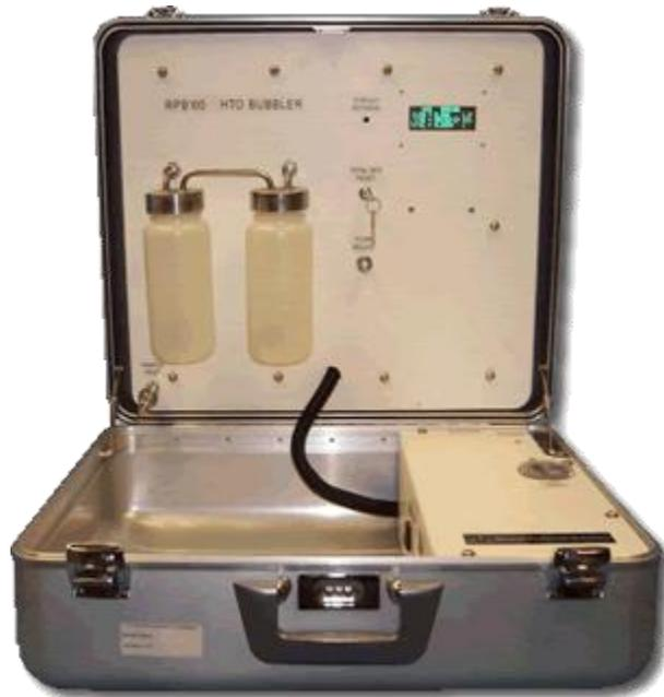
The RPB100 Portable HTO Bubbler is a two-vial, single stage bubbler designed for emergency response and short-term sampling applications. It is a complete HTO collection system contained in its own custom carrying case.
