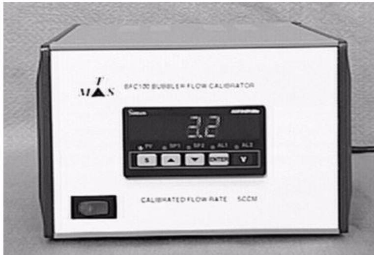
The BFC100 Bubbler Flow Calibrator provides the convenient and cost effective solution to the calibration of Bubbler flow controllers. In-situ calibration provides NIST traceability, minimal down-time, and cost savings. The Bubbler and the flow controller stay in place; therefore, the costs of down-time, Bubbler service technician time, calibration service, and shipping/handling are eliminated.
